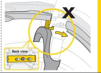
When installing DeFender M1 with suspension forks, make sure no part of the fork comes in contact with the DeFender M1 during its travel length. Otherwise damage to your bike or DeFender M1 may occur and it may also cause bodily injury.
